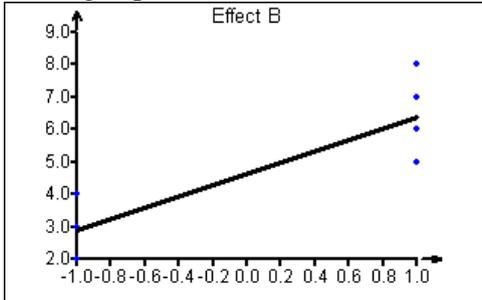
Averages plot gives average response for low and high level of each factor. The scale on all plots are the same so the plots can be compared.
