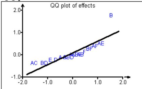
If all effects and interactions are zero, the effects distribution follow the normal distribution. In QQ-plot we can see deviations from normal distribution for individual factors. Such deviations (like factor B on the picture) can be interpreted as significant effect of the factor.
