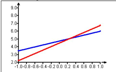
Interactions plot can reveal possible significant interactions of the first order between factors. Interaction will be diagnosed if the slopes of the blue and red line differ significantly. The scale on all plots are the same so the plots can be compared.
