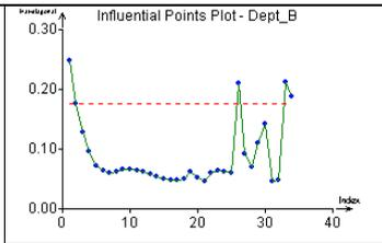
Plot of the projection matrix  $\mathbf{H}=\mathbf{X}(\mathbf{X}^T\mathbf{X})^{-1}\mathbf{X}^T$  diagonal elements. ( $\mathbf{X}$  is the matrix of the first partial derivatives w.r.t. the model parameters). The points plotted above the red horizontal line are considered to be potentially influential.
